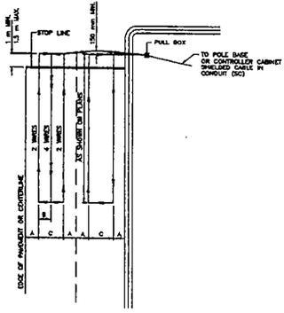
**LARGE LOOP DETECTOR INSTALLATION DETAIL**
