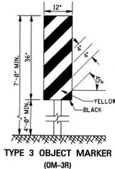
1. TYPE 3 OBJECT MARKERS SHALL BE USED AT ALL EXPOSED BRIDGE ABUTMENTS AND AT OTHER LOCATIONS AS DEEMED NECESSARY BY THE ENGINEER.
