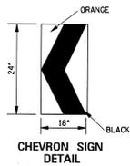
1. A CHEVRON SIGN CONSISTS OF A BLACK CHEVRON TYPE MARKING ON AN ORANGE BACKGROUND AND SHALL POINT IN THE DIRECTION OF TRAFFIC FLOW.
