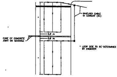
**TYPICAL DETAIL OF LOOP DETECTOR WHERE TRANSVERSE CONCRETE JOINTS, MANHOLES, ETC. ARE ENCOUNTERED**
