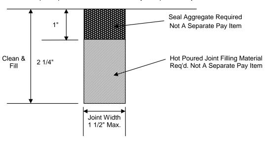
Variable Depth Asphalt-Remove as necessary to expose PCC joint
