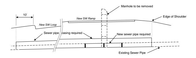
Detail of Sewer Pipe Encasement & Manhole Modification Near Gallatin Street
