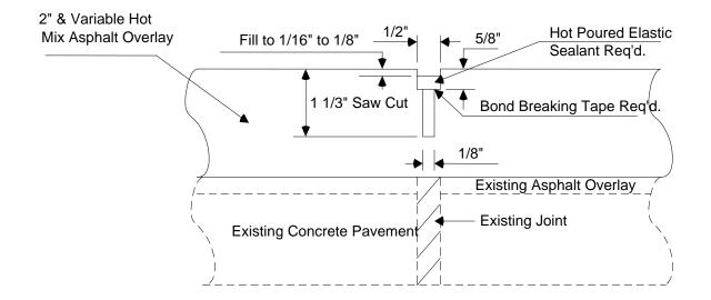
**DETAIL OF SAWING AND SEALING TRANSVERSE JOINTS**
