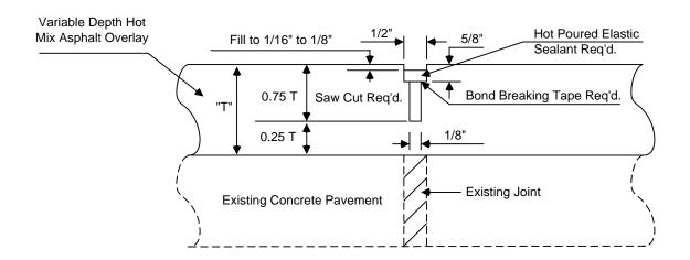
DETAIL OF SAWING AND SEALING TRANSVERSE JOINTS IN ASPHALT OVERLAY
