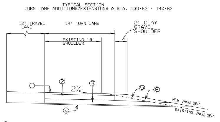
REMOVE EXISTING DBST OR HMA FULL DEPTH. SURFACE LIFT IS 2" HMA,12.5 MM MIX MT
