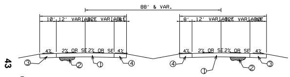
①MILL 1 1/2" AT CENTERLINE AND 2" AT EDGE OF PAVEMENT IN TANGENT SECTIONS AND 2" IN SE SECTIONS. INLAY WITH 2" 12.5 MM MIX, MT. LEVELING REQUIRED AS DIRECTED BY ENGINEER.
