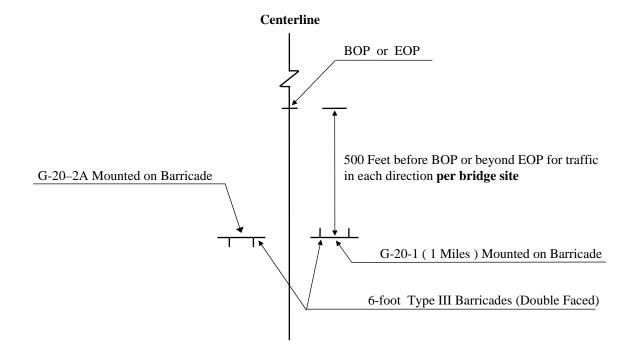
All Construction signing is included in the bid for Pay Item 618-A, Maintenance of Traffic. Fluorescent orange sheeting shall be used on all construction and traffic control signs except for R4-1 and R4-2 signs which shall be black legend and border on white background.
