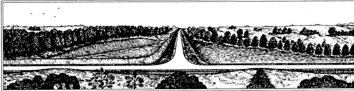
PERSPECTIVE OF TYPICAL DAYLIGHTING AT INTERSECTION IN CUT AND FILL
