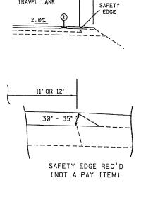
**OVERLAY** 11' OR 12' PAVEMENT WITHOUT TRENCH WIDENING
