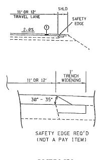
OVERLAY 11' OR 12' PAVEMENT WITH TRENCH WIDENING
