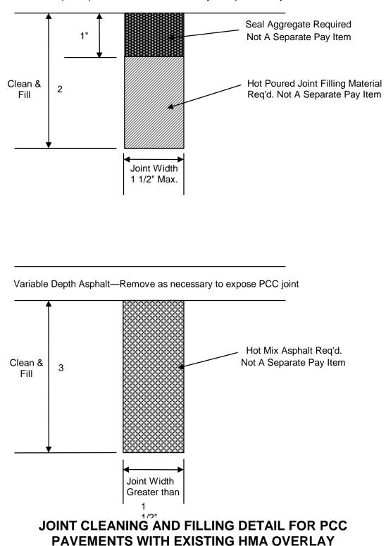
Variable Depth Asphalt-Remove as necessary to expose PCC joint
