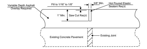
**DETAIL OF SAWING AND SEALING TRANSVERSE JOINTS**
