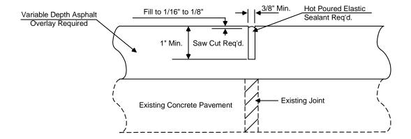
**DETAIL OF SAWING AND SEALING TRANSVERSE JOINTS**
