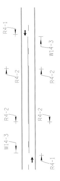
THE R4-1, DO NOT PASS SIGNS, SHALL BE PLACED ON THE RIGHT SIDE OF THE ROAD AT THE BEGINNING OF THE NO PASSING ZONE, ADDITONAL R4-1 SIGNS SHALL BE PLACED RIGHT AND LEFT IN INCREMENTS OF 750' TO 1000'. THROUGHOUT THE LENGTH OF THE NO PASSING ZONE.
