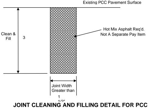
PAVEMENTS WITHOUT EXISTING HMA OVERLAY
