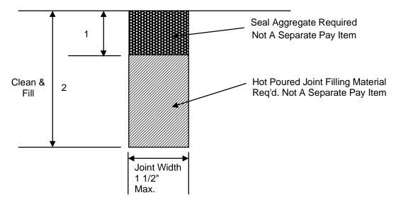
Variable Depth Asphalt—Remove as necessary to expose PCC joint
