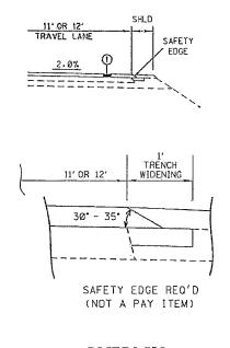
**OVERLAY** 11' OR 12' PAVEMENT WITH TRENCH WIDENING
