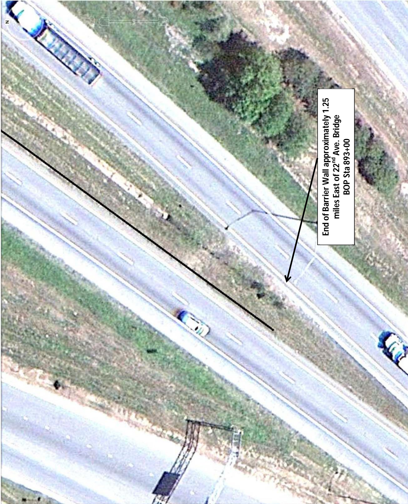
Cable Rail Location Detail I-20/I-59 from SR 19/SR 39 Interchange to Dees Rd. Lauderdale County
