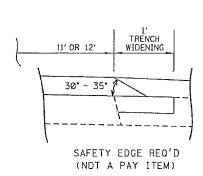
OVERLAY 11' OR 12' PAVEMENT WITH TRENCH WIDENING
