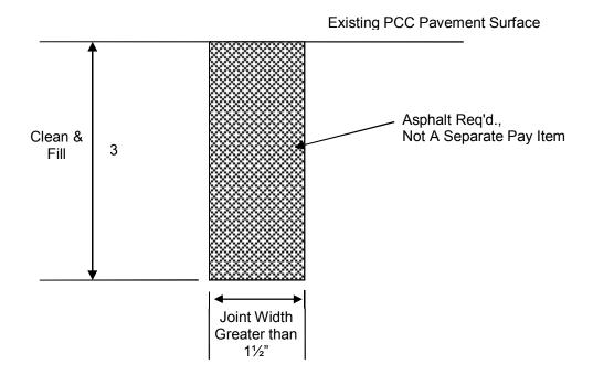
JOINT CLEANING AND FILLING DETAIL FOR PCC
