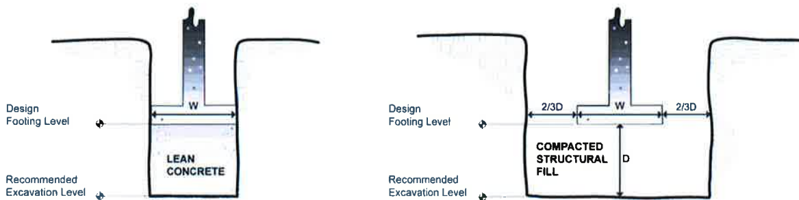
Lean Concrete Backfill
