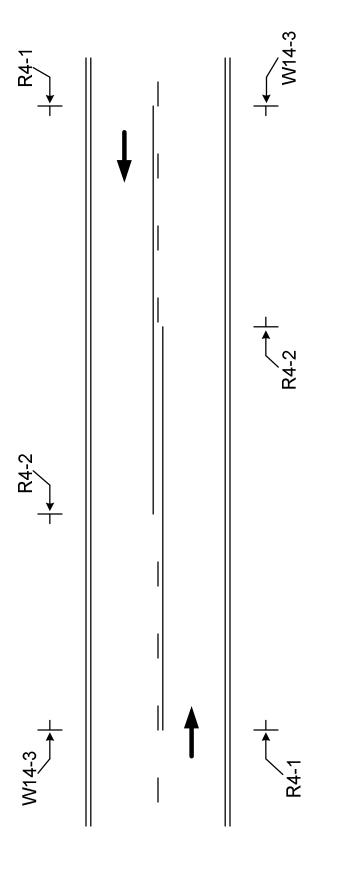
The W14-3, No Passing Zone sign, shall be placed on the left side of the road at the beginning of each no passing zone.
