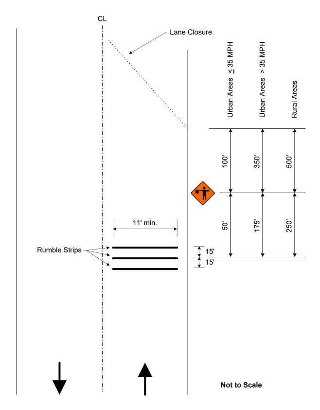
**Detail of Temporary Portable Rumble Strips**
