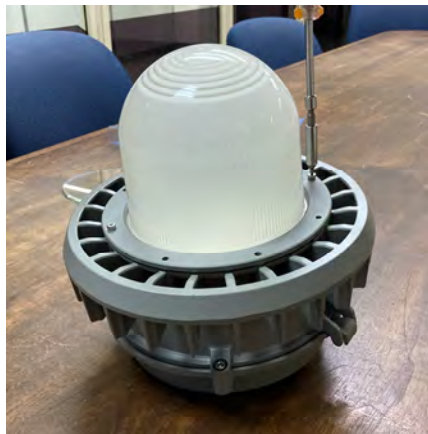
Step 7. If also using the dome guard, replace 4 pcs M4*16 screws, leaving one hole empty between each one. If not using the dome guard, replace all 8 pcs M4*16 screws
