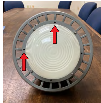
Step 7. If also using the dome guard, replace 4 pcs M4*16 screws, leaving one hole empty between each one. If not using the dome guard, replace all 8 pcs M4*16 screws
