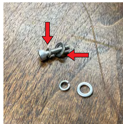
Step 9. Using the remaining 4 pcs M4*16 screws, 4 pcs small locking washers and 4 pcs larger washers (as shown), secure dome guard by tightening screws into 4 remaining holes.
