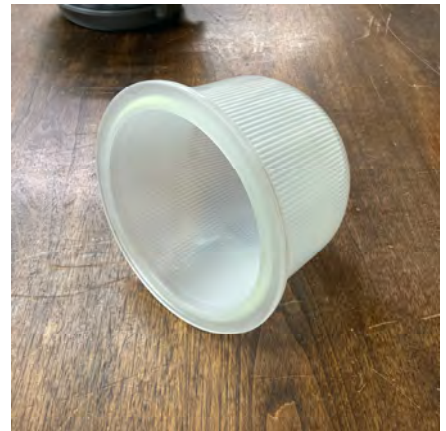
Step 4. Clean dome lens with wet wipe or wet cloth
