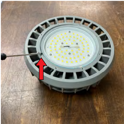
Step 3. Gently pry glass lens off using a flat screwdriver
