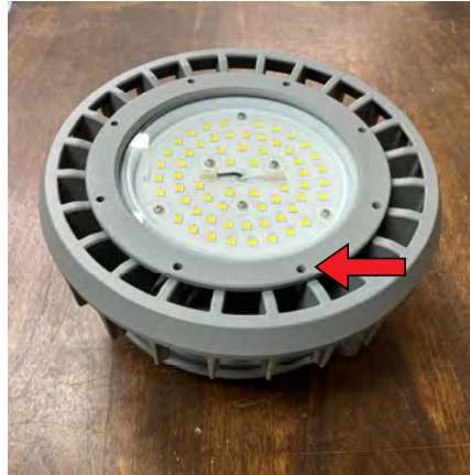
Step 1. From standard fixture with glass lens, remove 8 pcs M4*16 screws holding outer plate and glass lens on
