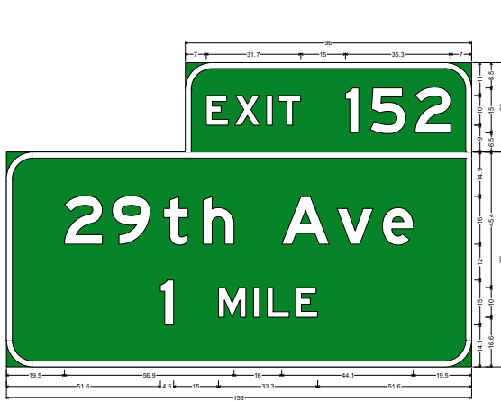
9.0" Radius, 2.0" Border, White on, Green; "EXIT", E Mod; "152", E Mod; 9.0" Radius, 2.0" Border, White on, Green; "29th Ave", E Mod; "1", E Mod; "MILE", E Mod;
