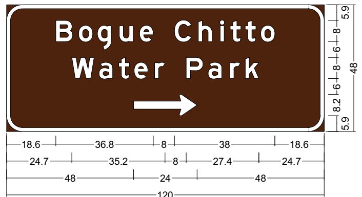
5035, US98, Pike ; 6.0" Radius, 1.5" Border, White on, Brown; "Bogue Chitto", E Mod; "Water Park", E Mod; Standard Arrow Custom 24.0" X 8.0" 0°;
