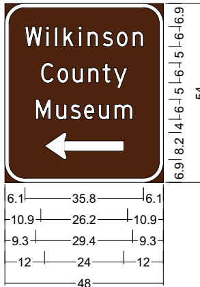
7016 US61 Wilkinson; 6.0" Radius, 1.3" Border, White on, Brown; "Wilkinson", D 85% spacing; "County", D 70% spacing; "Museum", D 70% spacing; Standard Arrow Custom 24.0" X 8.0" 180';
