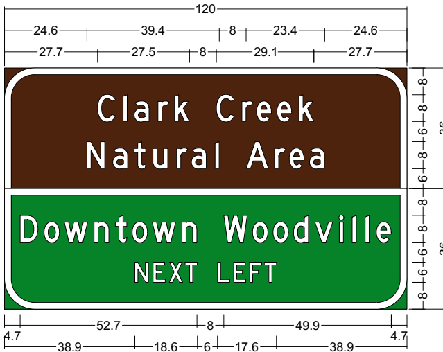
7021 US61 Wilkinson; 9.0" Radius, 2.0" Border, White on, Brown; "Clark Creek", D; "Natural Area", D; 9.0" Radius, 2.0" Border, White on, Green; "Downtown Woodville", D; "NEXT LEFT", D;
