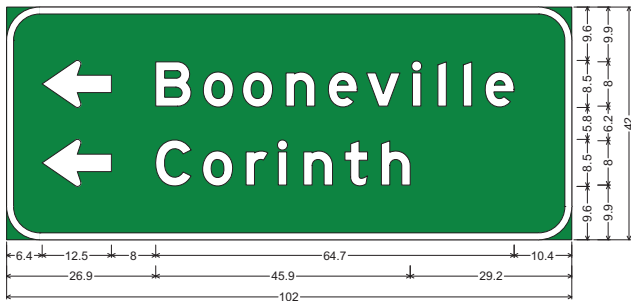
6.0" Radius, 1.3" Border, White on, Green; Standard Arrow Custom 12.5" X 8.5" 180"; "Booneville", E Mod; Standard Arrow Custom 12.5" X 8.5" 180"; "Corinth", E Mod; Table of letter and object lefts
