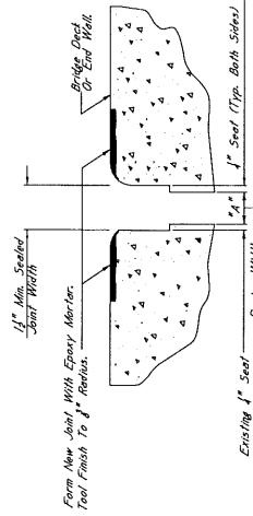
TYPICAL SECTION AT SAWCUT & JOINT REPAIR
