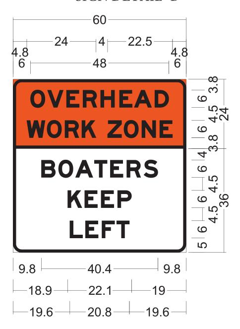
3.0" Radius, 1.0" Border, Black on, Orange; "OVERHEAD", E Mod 2K; "WORK ZONE", E Mod 2K 80% spacing;
