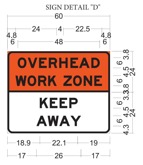
3.0" Radius, 1.0" Border, Black on, Orange; "OVERHEAD", E Mod 2K; "WORK ZONE", E Mod 2K 80% spacing;
