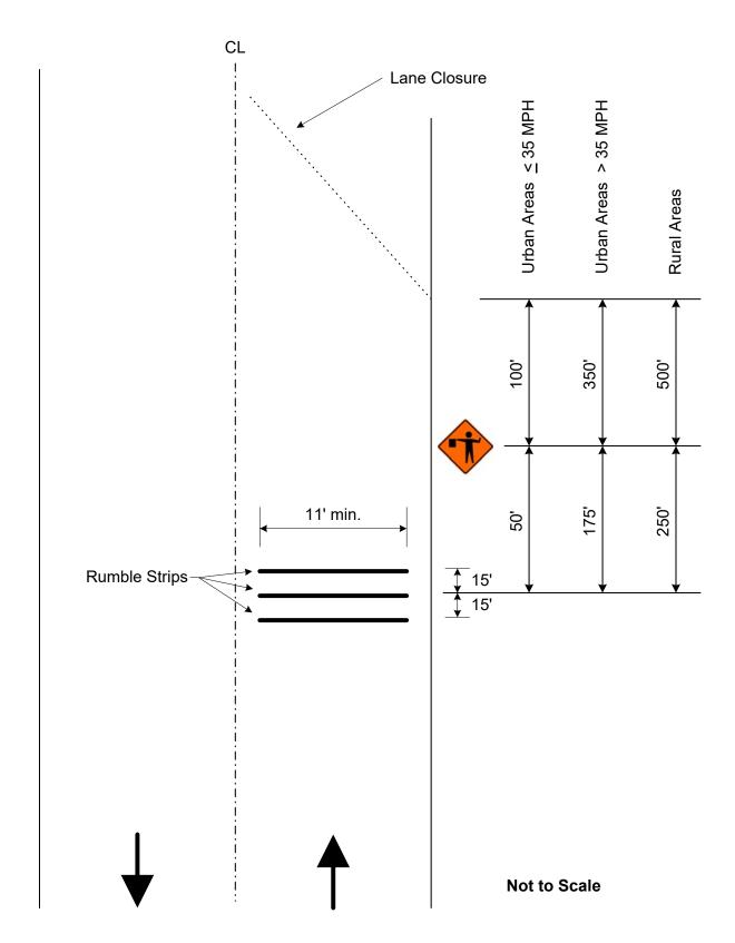
**Detail of Temporary Portable Rumble Strips**
