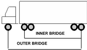
Maximum gross vehicle weight with maximum tandem axle weight of 44, 000 lbs.
