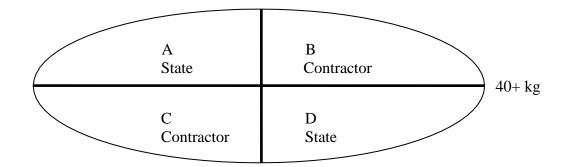
Combine diagonal quarters as indicated on the sketch to form the State sample (A & D) and the Contractor sample (B & C) for further quartering. Continue quartering process until test samples are in the oven. Place in a closed container and label the retained sample with the required information in Subsection 5.2.3.5 of this manual. Store samples in a safe place until no longer needed for sample verification.
