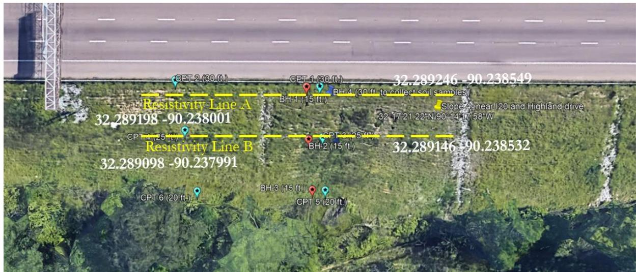
**Figure 4.25** Location of Slope 4, with ERI Test Lines
