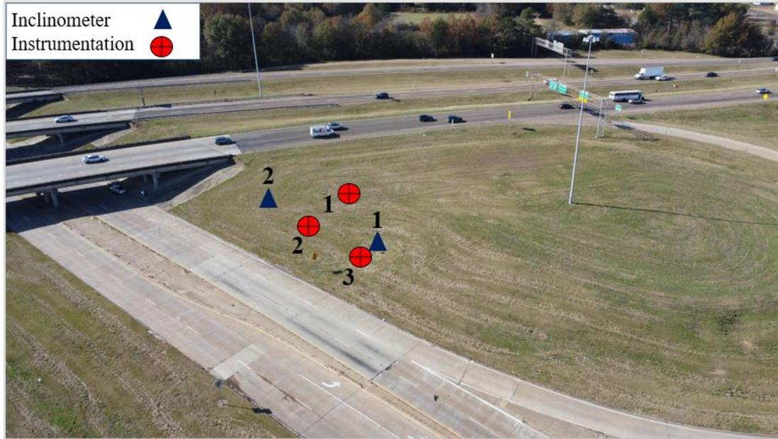
**Figure 3.24** Instrumentation Layout at I-Slope 3
