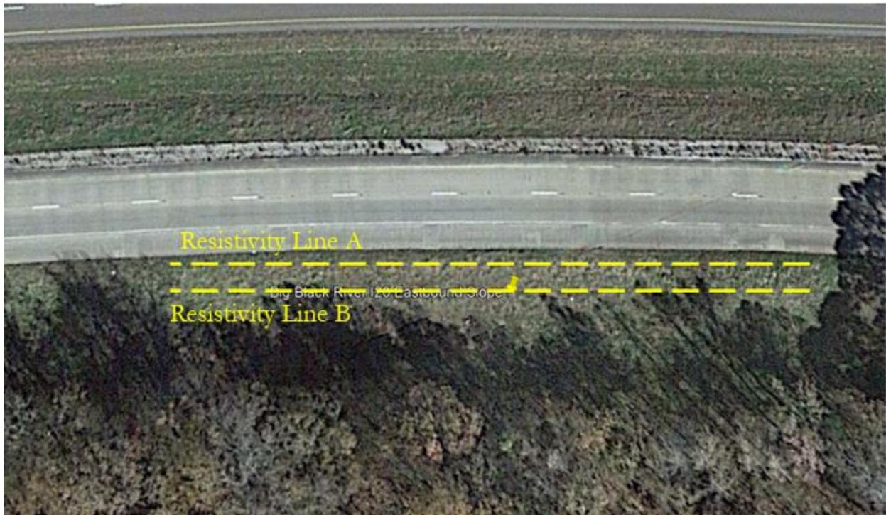
**Figure 4.94** ERI Test Lines in Failed Slope 12
