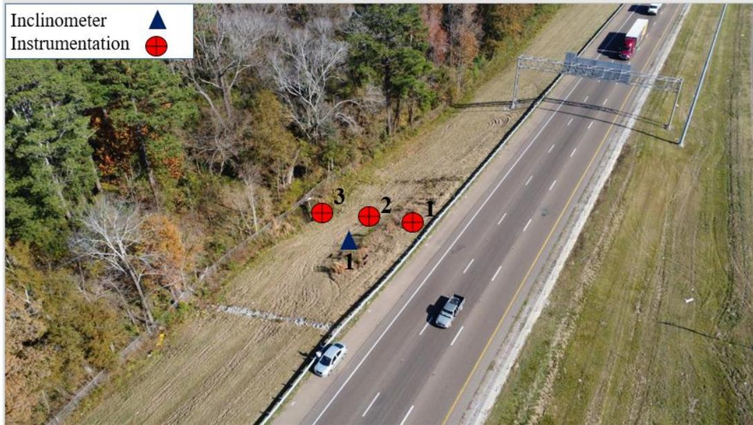
**Figure 3.34** Instrumentation and Inclinometer at I-Slope 4
