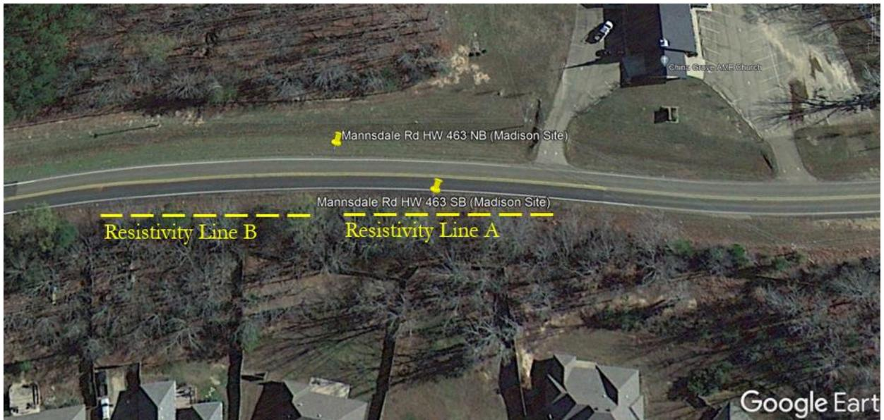
**Figure 4.121:** ERI Test Lines at Failed Slope 20
