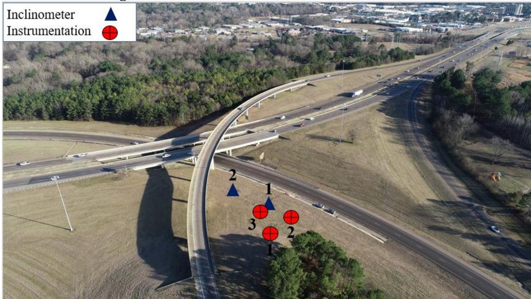
**Figure 3.4** Instrumentation Layout at I-Slope 1
