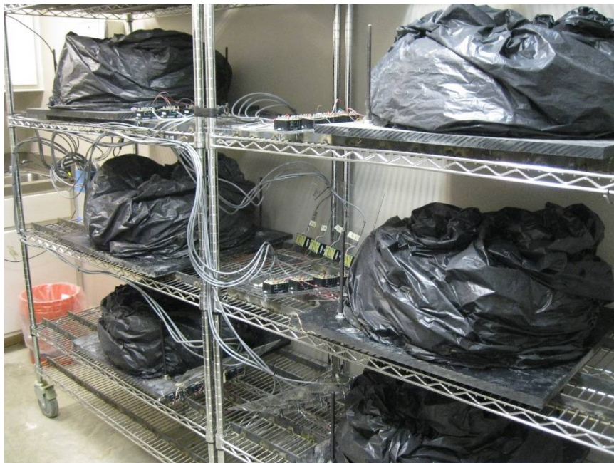
Figure 9. Cracking Tendency Specimens in Curing and Test Room
