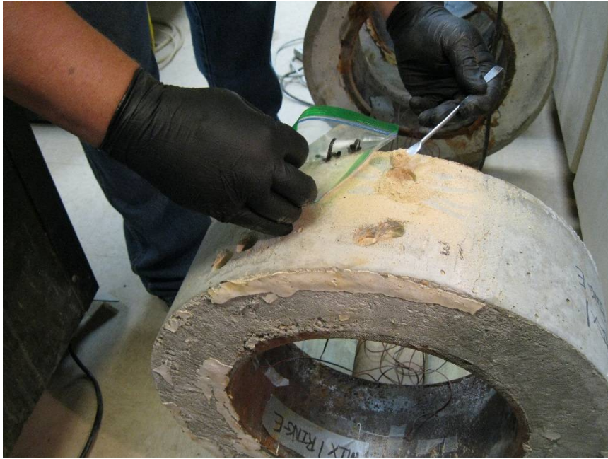
Figure 18. Collecting Powered Samples for Chloride Ion Analysis
