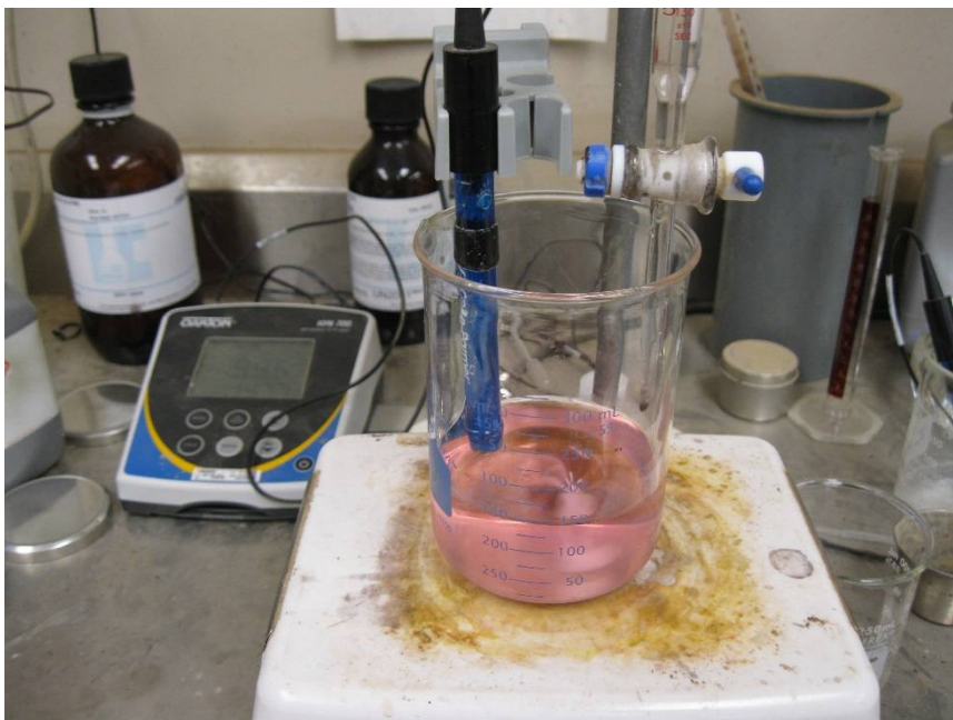
Figure 22. Titrating and Millivolt Reading of the Chloride Ion Sample
