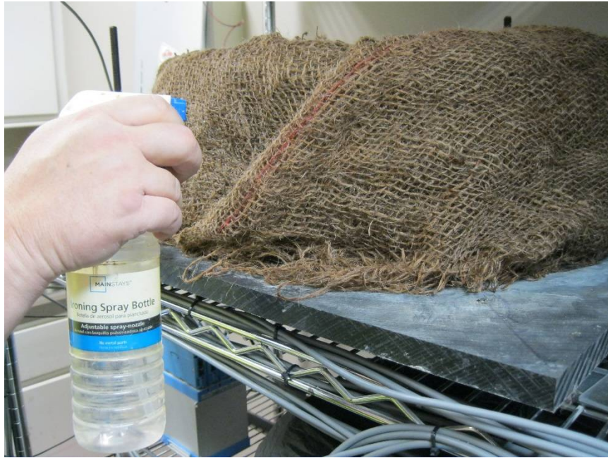
Figure 10. Wet Curing of Cracking Tendency Specimens
