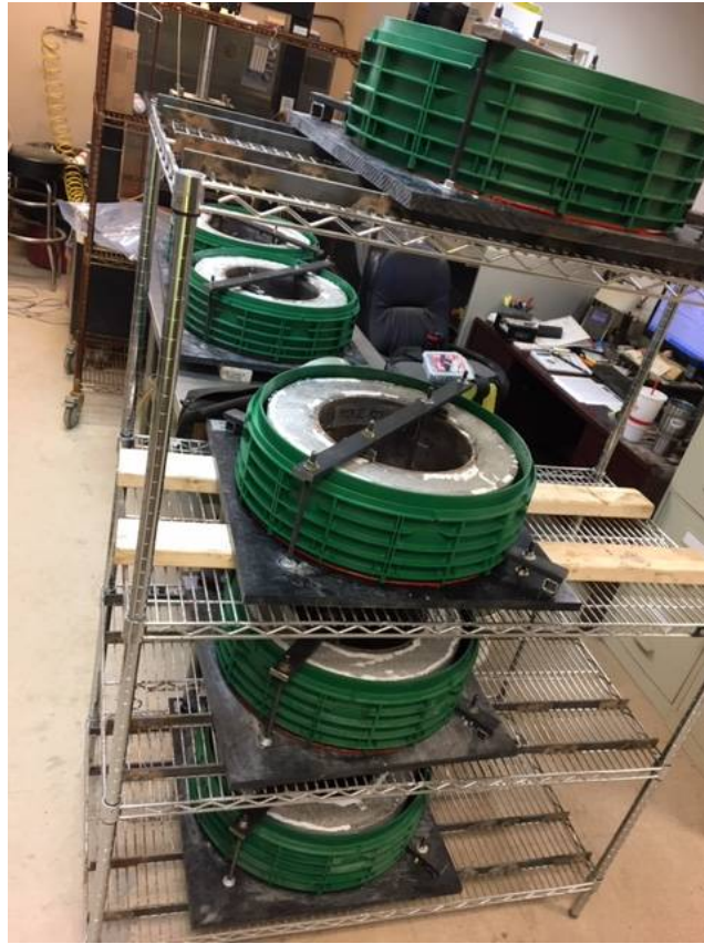
Figure 15. Apparatus for Ponding with Chloride-Rich Water
