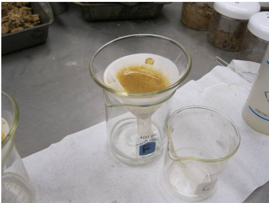
Figure 21. Filtering the Chloride Ion Sample
