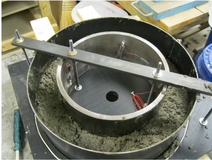
Figure 8. Molding of Cracking Tendency Specimens
