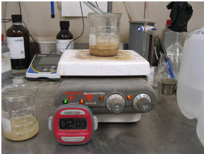
Figure 20. Boiling of the Chloride Ion Sample
