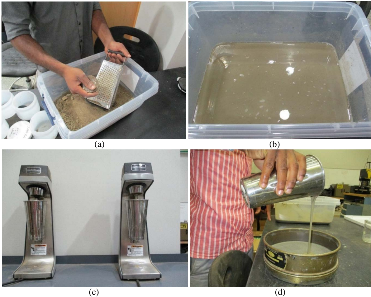
Figure 2.16 Sample preparation from the slurry mix to fully soften shear strength, (a) Shredding (b) Slaking (c) Blending and (d) Sieving
