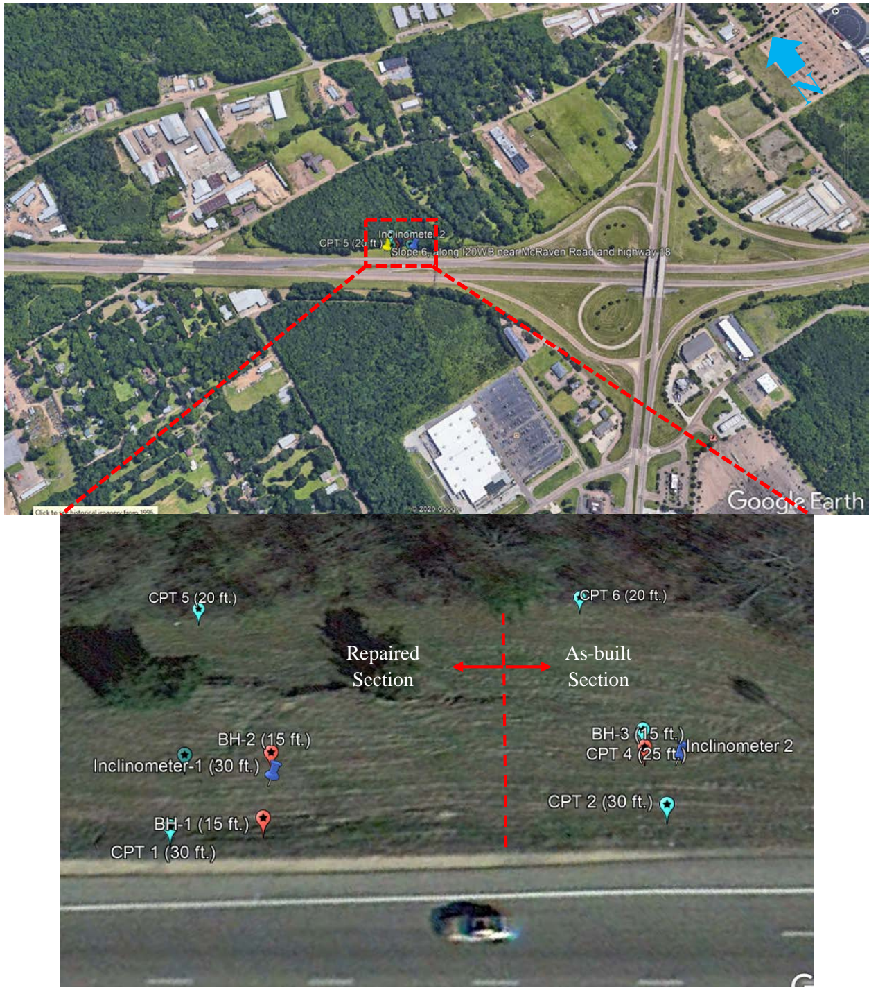
Figure 3.40 Location of CPT at Slope 6
