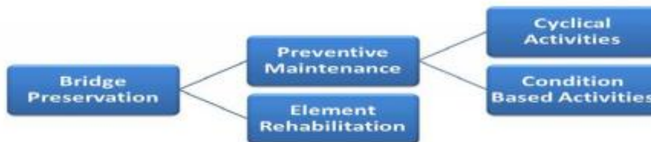
Figure 1 WisDOT Bridge Preservation Actions
