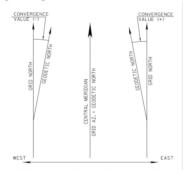
GEODETIC AZIMUTH = GRID AZIMUTH + CONVERGENCE
